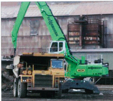
Sennebogen's standard design with guarded catwalks, railings and safety cameras inspired MCM Management to retrofit its entire equipment fleet to a similar standard.
